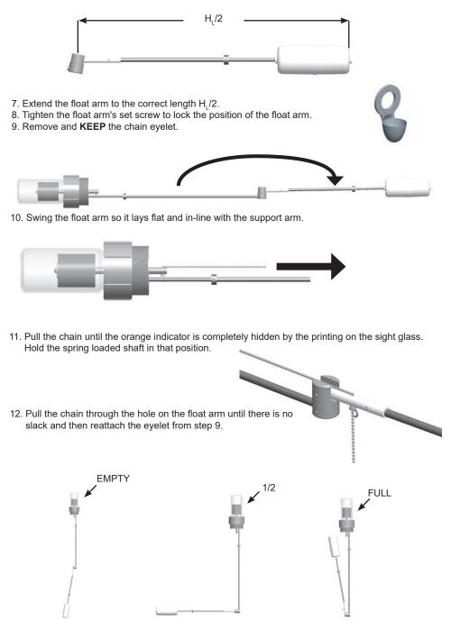
13. Verify proper function. If it's not working properly and if the orange indicator reads incorrectly, adjust the position of the eyelet. If repositioning the eyelet doesn't work, verify the length of the arms and overall length is correct.
