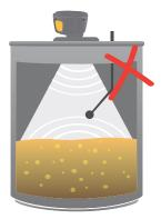
Install clear of manual gauges such as floats
