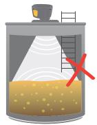
Install clear of stairs and other internal structures
