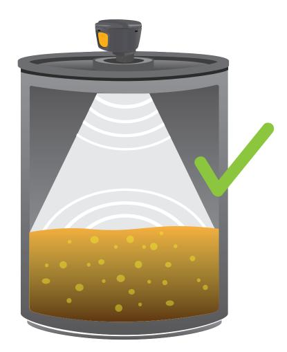
Ultrasonic sensors require an unobstructed column of air for precise measurement.
