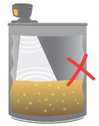
Install clear of welding seams and corrugated tank walls
