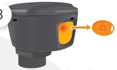
Remove the magnet when red light starts blinking.
