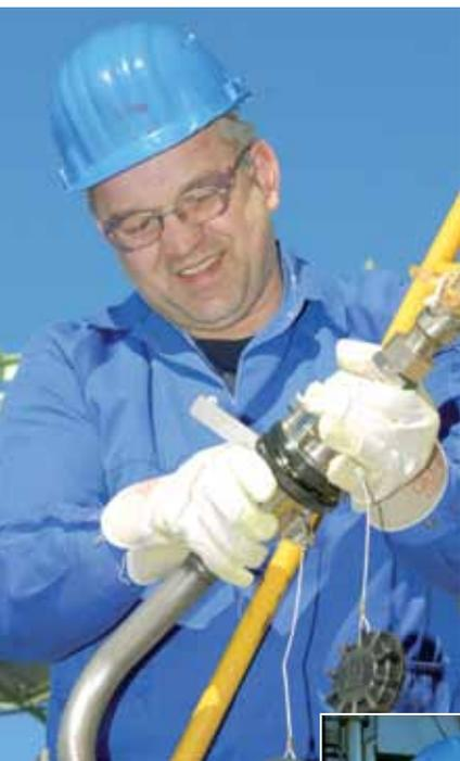
**Connected with a flick of the wrist: The gas displacement line is connected safely and in seconds to the TK series of dry disconnect couplings from RS (DN 25 width). Automatic safety locks ensure that decoupling is impossible when the valves are open, and that the coupling halves are closed during uncoupling.**
