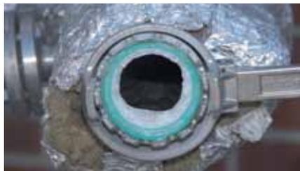
**Heating and thermal insulation are compulsory: The solidification point of the raw material is around 90 °C.**
